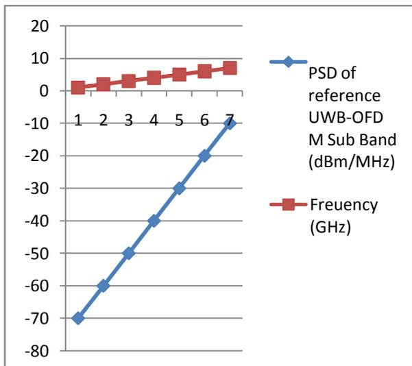
Fig: 5. Measured spectrum of reference UWB-OFDM sub band
