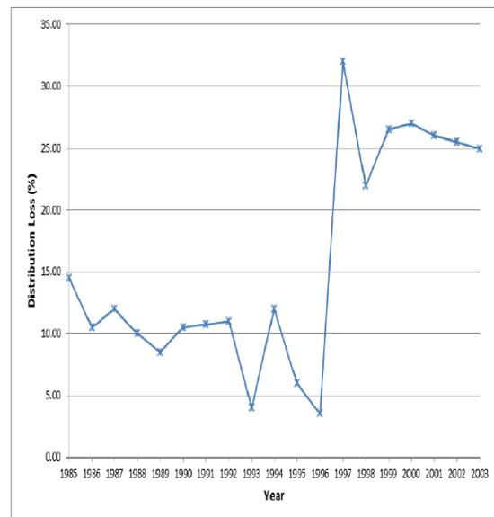
Fig: 1. Total Distribution Losses of ECG, 1985-2003
