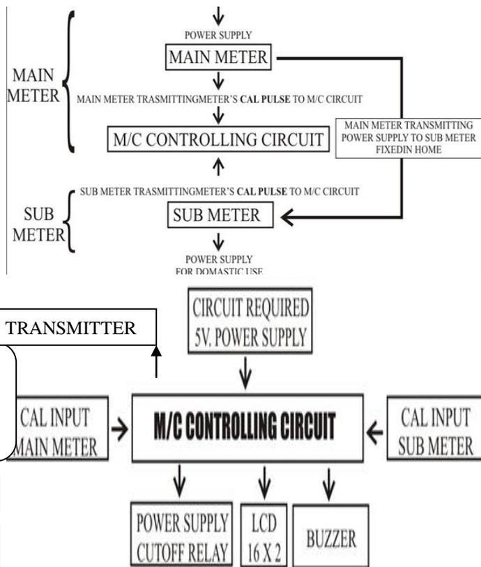
Our circuit is working on 5v power supply, which is regulated by regulator 7805. We are using 12v. Step down transformer for circuit. The calibrating pulse is given as an input to microcontroller from both meters. If any meter is tampered, the pulse from one of the meter is disturbed in this case the relay cut the supply within 1 minute and this information is transmitted to nearest substation.
