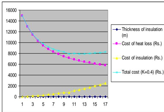
Fig. 3. Variation of cost with thickness of Corrugated Asbestos insulation
