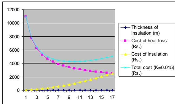
Fig. 4. Variation of cost with thickness of Polyurethane Rubber insulation (K=0.015)
