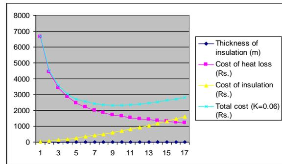
**Fig: 1.** Variation of cost with thickness of Rock wool insulation
