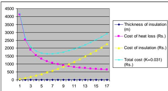
Fig. 5. Variation of cost with thickness of Cellular Plastic insulation (K=0.031)
