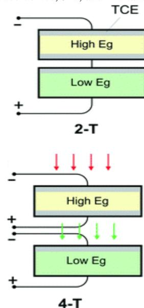
This way the individual devices from the stack can be fabricated independently, thereby also significantly expanding the processing
