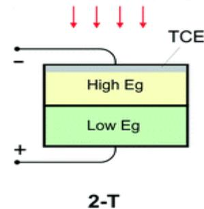
This is the configuration almost exclusively used in commercial products because it involves a minimum number of processing steps, substrates, layers and interconnections. [11-12]
