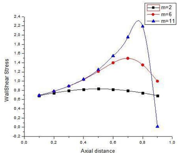
**Fig. 4:** Variation of wall shear stress with axial distance for  $\alpha = 90^\circ$ ,  $C = 0.5$  different values of  $m$
