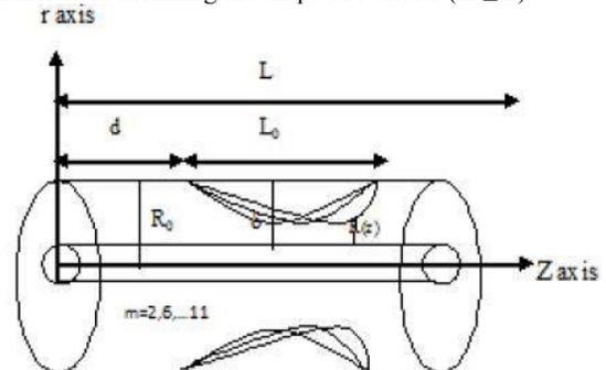
Fig-1: Geometry of an axially non-symmetric stenosis in an artery
