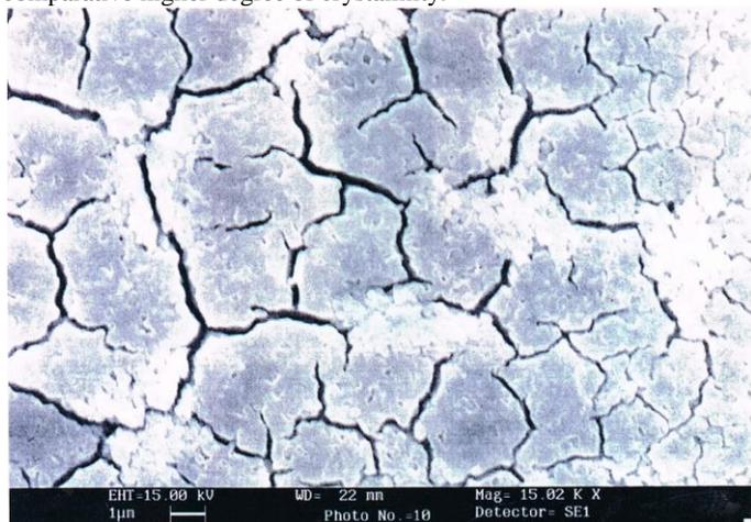
**Fig.1.** SEM image of CdS thin film on to glass substrate.
