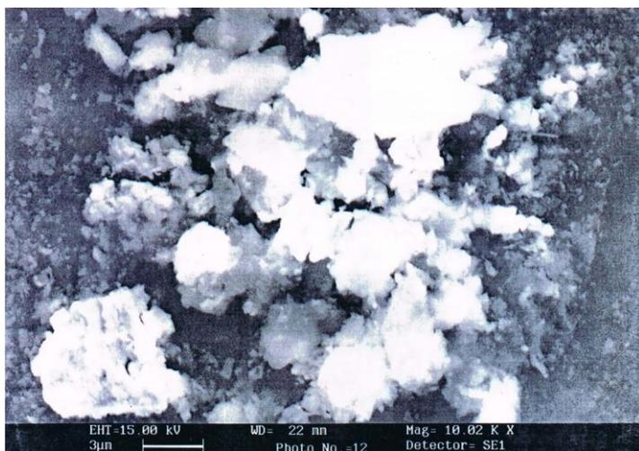
**Fig.2** SEM image of Pani/CdS thin film on to glass substrate
