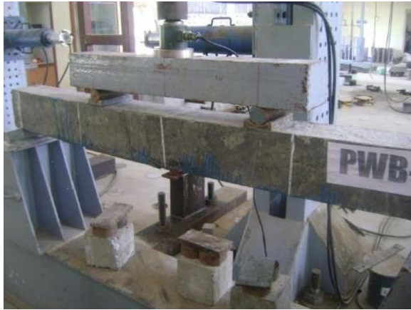
Fig 7. Crack patterns observed in partially wrapping beam
