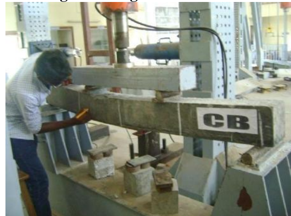
Fig 5. Deflection and Crack patterns observed in control beam under loading
