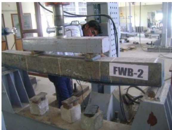
Fig 9. Crack patterns observed in fully wrapping beam
