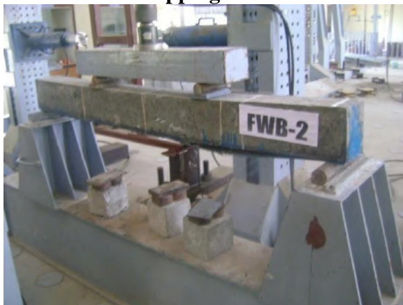
Fig 8. CFRP fully wrapped on its tension zone
