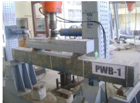
Fig 6. CFRP partially wrapped on its tension zone
