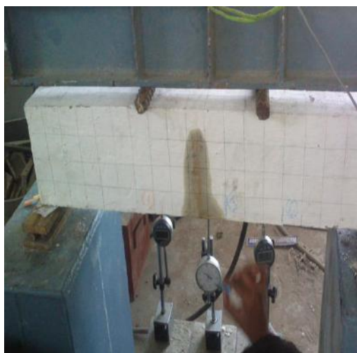
Fig 5.1 Beam arrangement for load deflection test
