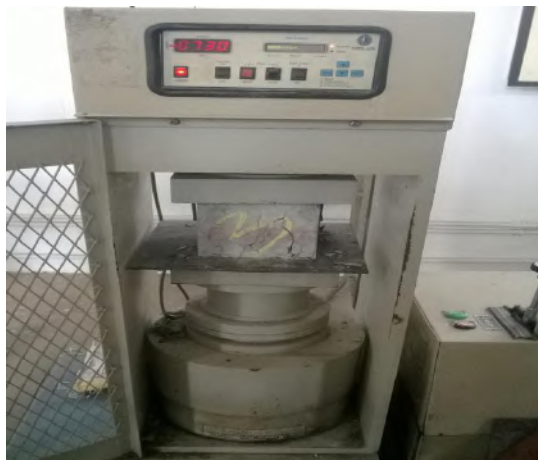
Fig 2.1 Compression test for first specimen
