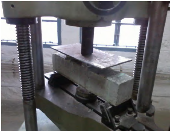
Fig 2.5 Specimen arrangement for Flexural strength test
