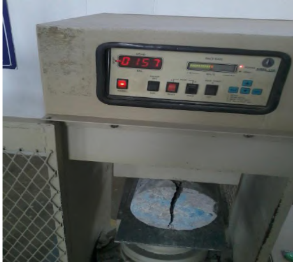
Fig 2.4 Split tensile test for first specimen
