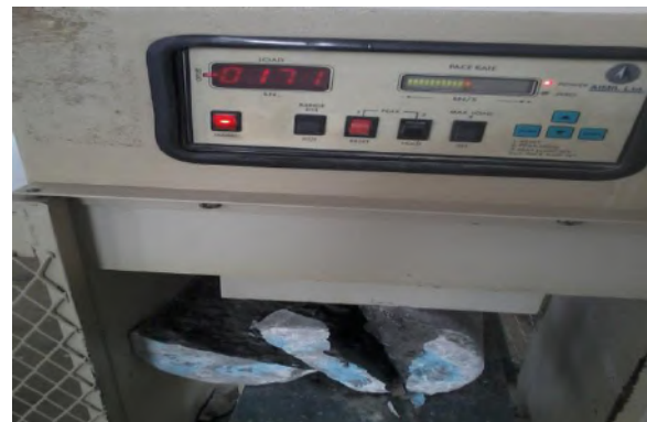
Fig 2.3 Split tensile test for first specimen
