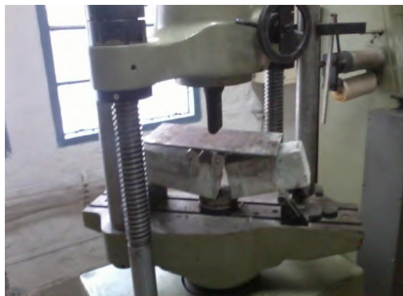
Fig 2.6 Flexural strength test
