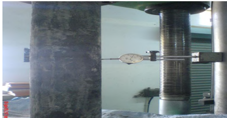
Figure: 3 Test setup for RC column
