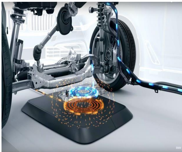
Fig: Wireless power transmission between transmitter and receiver coils.
