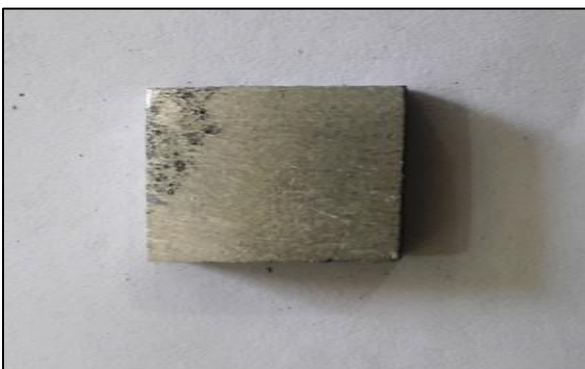
Fig 9: MMC sample prepared for hardness test
