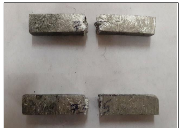
Fig10: MMC sample After Toughness Testing
