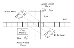
Fig. 1: Block diagram of Indian railway gate crossing.
