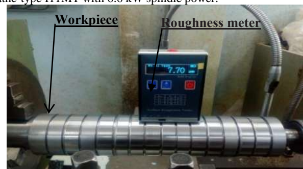
Fig.1 Experimental setup for roughness measurements. The measurements of surface roughness ( R_a ) for each cutting condition were obtained from KR-100 roughness meter. The length
